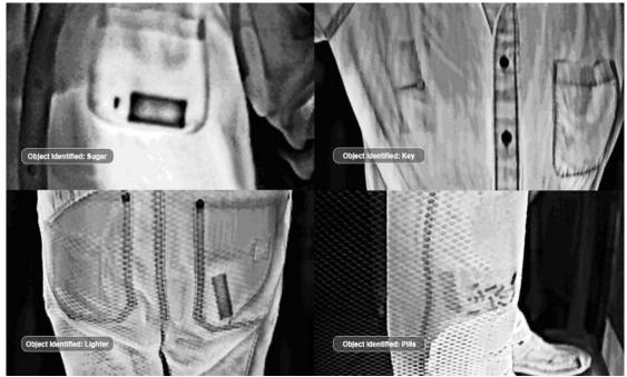
Objects as detected through **thermo-conductive imaging**. 3D-printed objects are just as clearly detected using the same technology, as well as via **backscatter x-ray** and **millimeter-wave scanners**.
